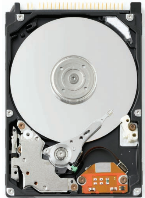
▲ Figure 3.3 Hard disk drive – the hard disk (platter) is the media and the hard disk drive (HDD) is the storage device
