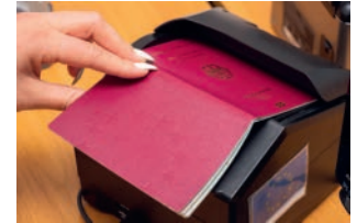
▲ Figure 2.23 Using OCR to process a passport
