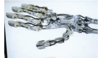
▲ Figure 6.24 This is an example of prosthetic arm produced by 3D printing. Such technology can be life-changing to an amputee.
